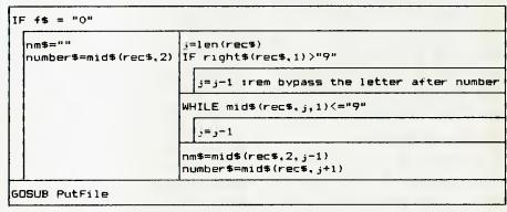
Figure 5. The logic of the 'RealRecord' module.
